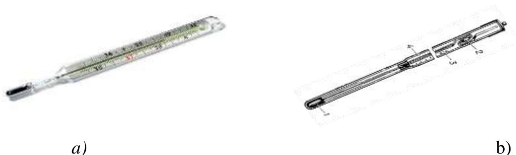
**12-rasm.** a-simobli termometr, b-metastatik termometr: 1-rezurvar, 2-qo ‘shimcha kamera, 3- kamera, 4-asosiy shkala
